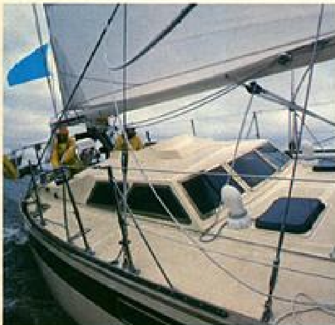
12 Lexan ports and double-barned hatches.
