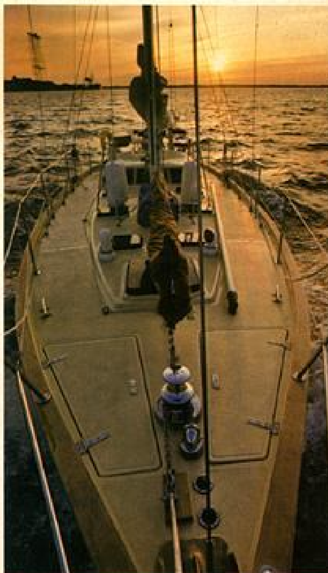
Flushdeck and foredeck sail lockers
