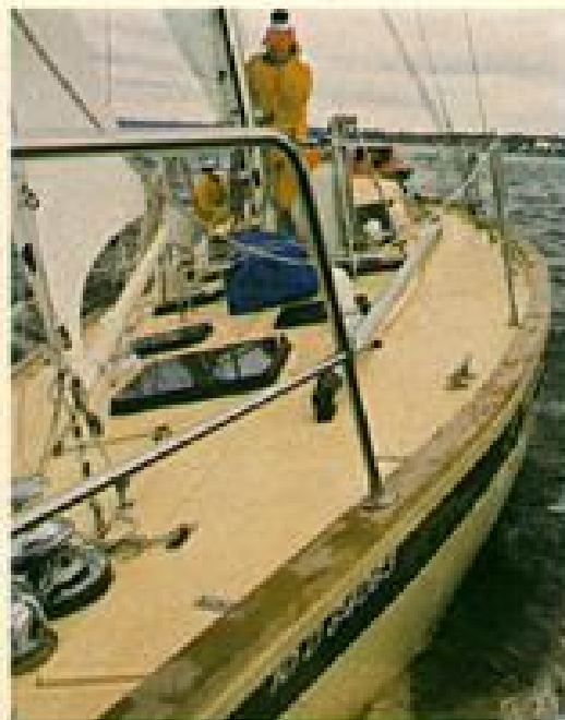
Flushdeck and mast pulpits
