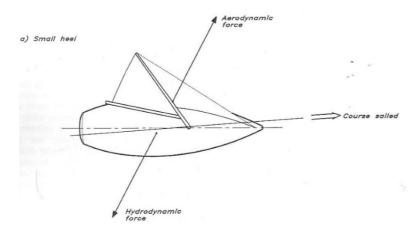
If the yacht heels more, due to the height of the aero forces / rotation axis of the boat heeling, the aero forces moves more leeward while the opposite is true for the hydro forces moving a bit winward, causing the forces to act on different lines and creating a turning moment in horizontal projection:
