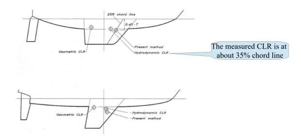
• Within the PYD method, Jean-Francois extends the keel to the real waterline for 14,000 kg (30,864 lbs), being a typical working displacement for a cruise. This would be the actual "hook weight" we would expect to be shown on a crane if the yacht were to be lifted out of the water in
