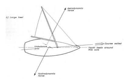
>>> Then, an extra hydro force provided by the rudder is required to recover the equilibrium, i.e. an extra lift at the cost of an extra drag. Moreover, upwind when the boat speed is already close to its maximum, the aero force due to more windspeed can increase more than the corresponding hydro force due boatspeed little or no increase. Up to a situation out of control when the rudder wing stalls and cannot provide more lift.
