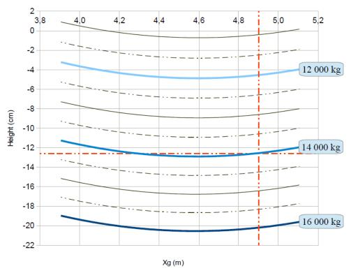
>>> Result of this example : Displacement 14 000 kg (the crossing of the red lines) at Xg 4,901 m, generating a trim of – 2,36°
