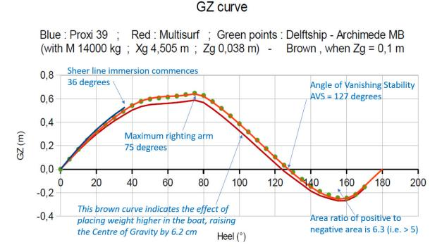
**Recommendations :** The study makes important assumptions regarding hull dimensions, displacements, and weight distribution. Therefore it is recommended that these assumptions are refined through a process of accurate measurement and an inclining test of a reference hull, plus reporting by owners of actual displacements by way of draft and "hook weight" information.
